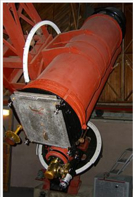
Tombaugh created his photographic plates using this 13-inch astrograph
