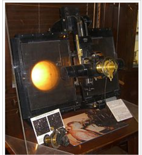
Tombaugh compared his photographic plates using this blink comparator.
